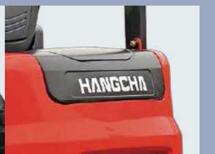
Easy opened counterweight cover is to protect the internal controllers to avoid water and dust
