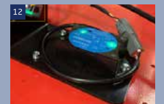
Angle sensor: when it is lifting and walking on the slope, the sensor will automatically judge the status of the machine, if the angle is larger than the rated angle, it will alarm to remind the operator.
