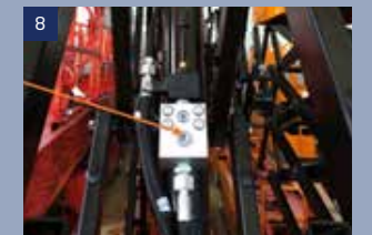
Explosion proof valve: To prevent the machine falling when the oil pipe is leaking
