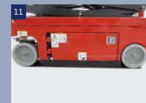
Anti-overturning system: When the machine raises to more than 6.5ft, this system will work automatically, to protect the machine from overturning while walking on un-leveling ground.
